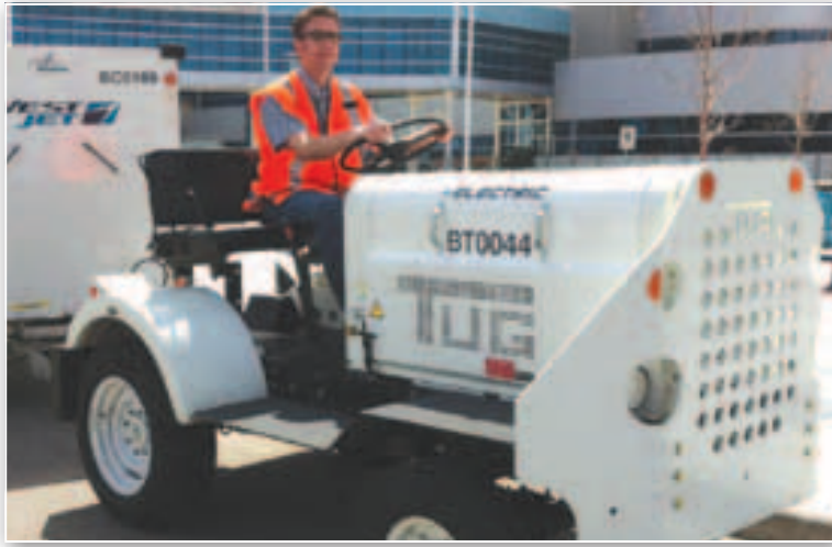
WestJetter Leigh Hoey sits atop WestJet's lithium polymer-powered baggage tug, developed in partnership with Corvus Energy of Richmond, BC. The technology allows the airline to transport baggage to and from the aircraft without the use of fossil fuels. (CNW Group/WestJet)
