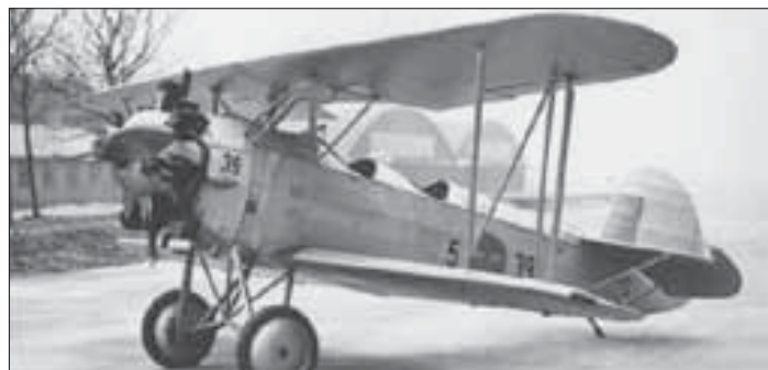
The Raab-Katzenstein RK-26 Tigerschwalbe was a German twin-seat biplane trainer aircraft designed by Gerhard Fieseler at the end of the 1920s. Primary users were the Swedish and Finnish Air Forces.
